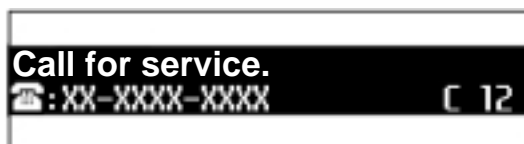
Figure 1-5-2 Service call code display
